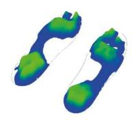
Foot pressure measurement: left balance shoe Sirius, right Pluto S
