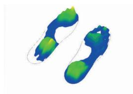
Foot pressure measurement: left balance shoe, right Uranus
