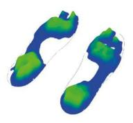
Foot pressure measurement: left balance shoe, right Pluto S
