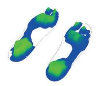
Foot pressure measurement: left balance shoe, right Merkur A
